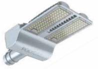
Highly efficient LED street light with 135lm/w having pressure die-cast housing, polycarbonate lens optics. IP 66 protection including driver, best solution for NHAI with high pole spacing. Equipped with 4kv internal & 10kv external surge protection.
