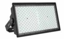
140lm/w LED floodlight luminaire with pressure die-cast housing having toughened glass cover with secondary lens optics, IP 66 protection including driver, 4 kV in-built and 10 kV external surge protection.
