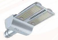
Highly efficient LED street light with 1351m/w having pressure die-cast housing, polycarbonate lens optics for better distribution. IP 66 protection including driver, best solution for NHAI with high pole spacing. Equipped with 4kv internal & 10kv external surge protection.
