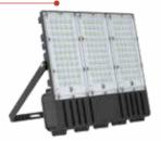
120lm/w LED floodlight luminaire with pressure die-cast housing having IP lens optics with IP 66 protection including driver, 4 kV in-built and 10 kV external surge protection.
