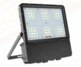
120lm/w LED floodlight luminaire with pressure die-cast housing having toughened glass cover with secondary lens optics, IP 66 protection including driver, 4 kV in-built and 10 kV external surge protection.
