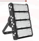
140lm/w LED floodlight luminaire with pressure die-cast housing having toughened glass cover with secondary lens optics, IP 66 protection including driver, 4 kV in-built and 10 kV external surge protection.
