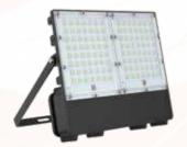
120lm/w LED floodlight luminaire with pressure die-cast housing having IP Lens optics with IP 66 protection including driver, 4 kV in-built and 10 kV external surge protection.
